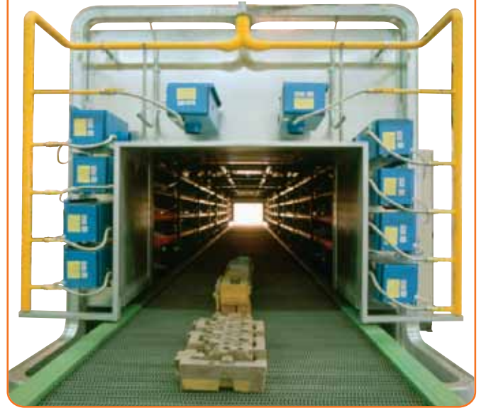
Example of a drying installation for water paintings on foundries souls.
